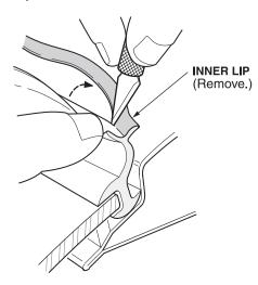
3. With an O-ring pick or similar tool, pull up the outer edge of the molding, and apply 3M Black Super Silicone Sealant under it, along the A-pillars and the upper edge of the windshield.
