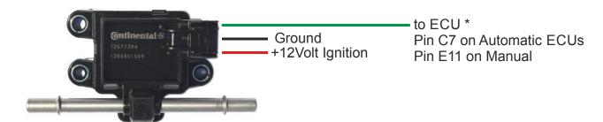
\* On a Automatic to Manual converted ECU, like the PND-A5x connect the Ethanol Content Sensor direct to Pin C7.
